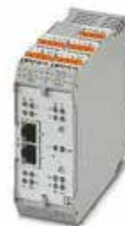
8 IO-Link ports, 8 digital inputs
