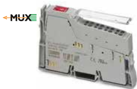
1/4 relay outputs, 5 - 253 V AC, gold contacts
