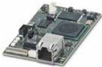
Embedded router/firewall with VPN
