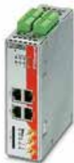
With firewall and VPN, integrated 4-port switch
