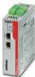
Router with simplified 2-click firewall and VPN
