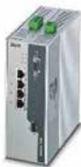
4 / 8 RJ45 PoE ports and 1 / 2 SFP ports
