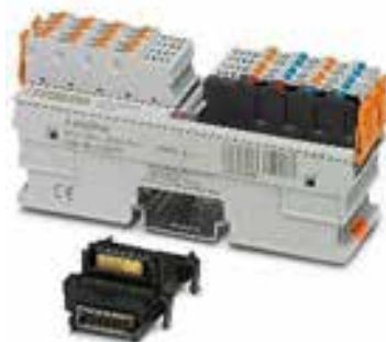
16 inputs and 8 outputs, 2 A
