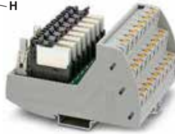
Digital input module with 8 channels for 24 V DC
