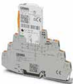
Double wire (loop), floating, 3/6 connection grounded via gas-filled surge arrester, with knife disconnection, e.g., for 4 ... 20 mA current loop
