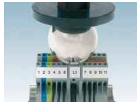
Back of hand safety Test ball with 50 mm diameter
