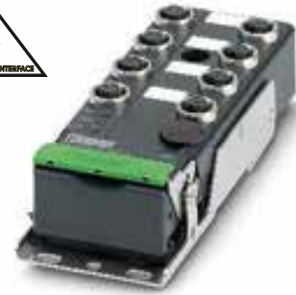
4 digital inputs and 4 digital outputs
