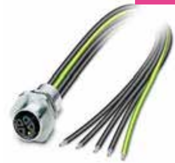
K-coded, cable cross section: 1.31 mm 2 , 4-pos.+PE
