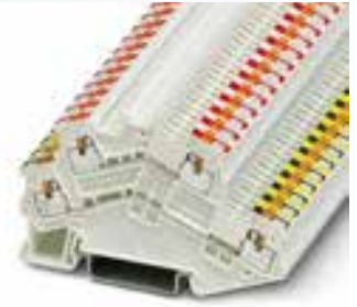
16 A, double-level terminal block, 4 connections, for KNX bus wiring
