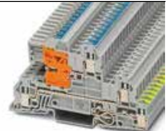
4 (4) mm 2 , 30 A, three-level terminal block, 1 x L phase conductor, 1 x N conductor can be disconnected, 1 x PE
