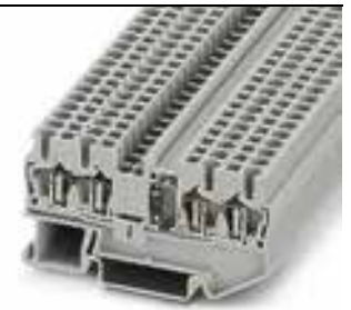
1.5 A, diode terminal block, 1N 5408 (1000 V/1.5 A), 4 connections
