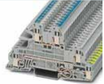
4 (4) mm 2 , 30 A, three-level terminal block, 1 x L phase conductor, 1 x N conductor, 1 x PE
