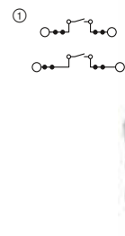
16 A, double-level terminal block with one disconnect knife per level, desk design
