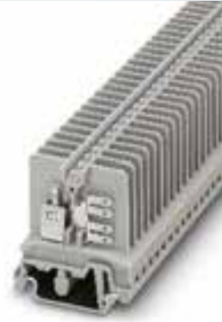
4 (4) mm 2 , 32 A, feed-through terminal block, with screw and slip-on connection
