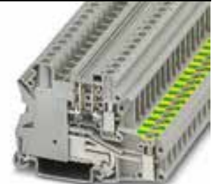
0.5 A, diode terminal block, 1N 4007 (1300 V/0.5 A), conducting direction: from right to left
