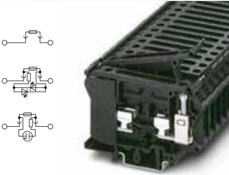
16 (16) mm 2 , 10 A, lever-type fuse terminal block for 6.3 x 32 mm cartridge fuses
