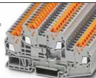
17.5 A, double-level diode terminal block, 1N 4007 (1300 V/0.5 A)
