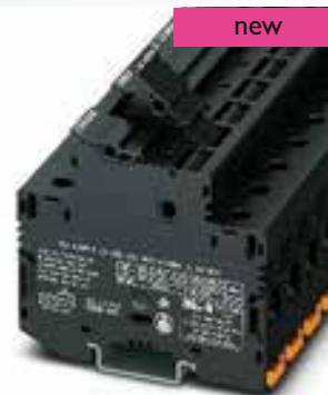
16 (25) mm 2 , 32 A, lever-type fuse terminal block for 10.3 x 38 mm midjet fuses
