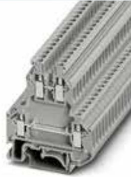
2.5 (4) mm 2 , 32 A, double-level terminal block
