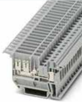
2.5 (4) mm 2 , 32 A, feed-through terminal block, with screw and slip-on connection
