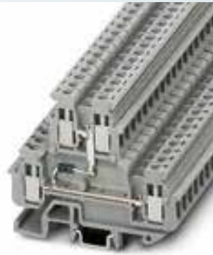
2.5 (4) mm 2 , 24 A, double-level terminal block, with built-in 1N 4007 diode
