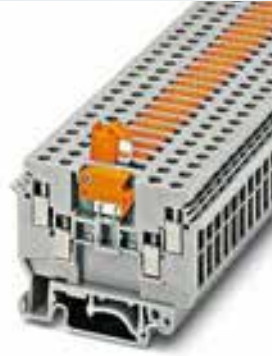
4 (6) mm 2 , 16 A, knife disconnect terminal block, 4 connections, with test socket screw
