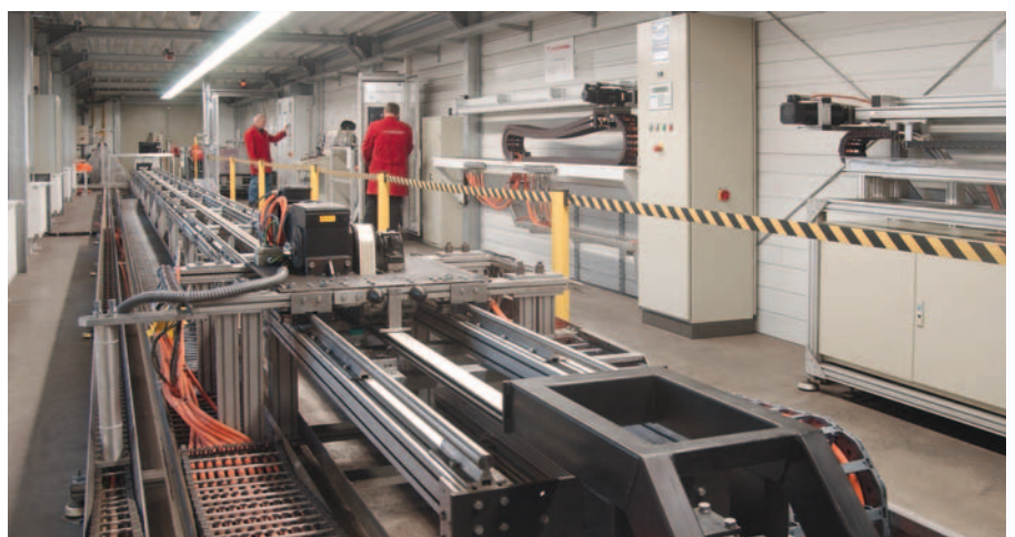
Drag chain test system
